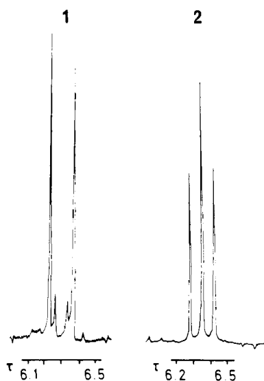
Figure 2. Comparison of the shapes of the OMe proton signals for the complexes 1 and 2 ( \text{R} = \text{OMe} ).
